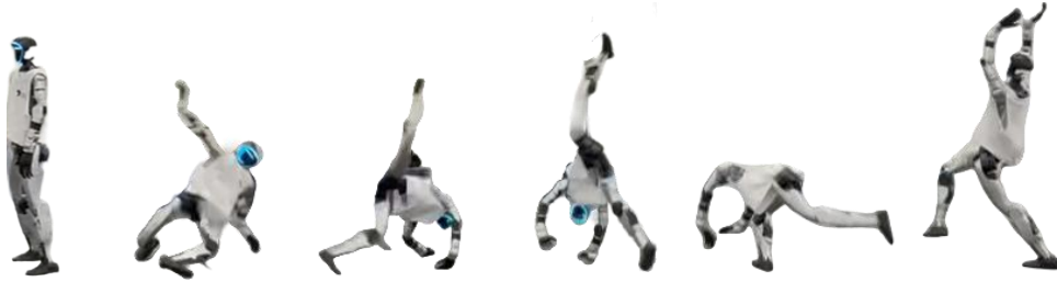
Figure 11: Injecting new agile skills (cartwheel) into a behavior foundation model. Our fixed inter-dataset sampling ratio stabilizes training and enables successful skill acquisition, whereas naive merged prioritized sampling leads to instability.
