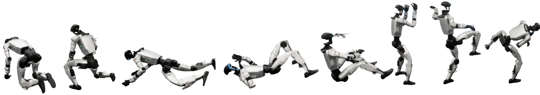
Figure 8: Goal reaching performance. UFO-TeCH enables flexible goal reaching by leveraging temporal-distance representations, allowing the policy to reliably reach target states from arbitrary initial configurations.
